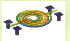
The current distribution and radiation pattern of a handset antenna modeled on IE3D
