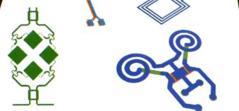
Ensemble allows you to design complex planar antennas and on-chip components like spiral inductors, vias and interconnects.
