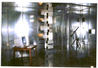
1. This mode-stirred chamber provides a tightly controlled environment for performing shielding-effectiveness measurements.
